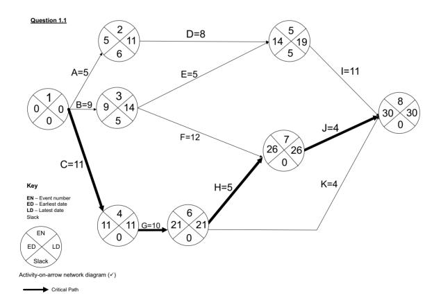
1.2 Write down the critical path(s) using the letters of the tasks and calculate and write down the duration of the project. How many paths are there in total? Identify them all and write them down.
