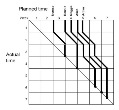
The timeline chart illustrates the way in which targets have changed through-out the duration of a project. Planned time is shown along the horizontal axis and actual time along the vertical axis. In the ideal situation (no delays), the Planned Time and the Actual Time will correspond on the diagonal.
